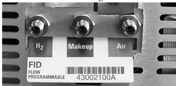
Figure 5. Gas line connections
